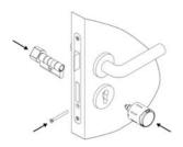
Insert the DoorLock-DC profile cylinder into the door and secure it with the supplied forend screw. Then push the electronic knob into the cylinder until the knob engages. To dismantle, use the disassembly card to loosen the connection between the profile cylinder and the knob. Then follow the steps above in reverse order
