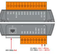
Connect the device with a patch cable to a PoE-capable switch or with a PoE injector to a switch without PoE.
