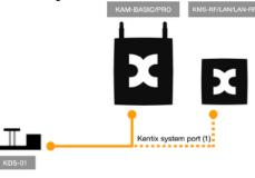
Connect the dust sensor to an AlarmManager or MultiSensor with a patch cable. Power is supplied directly from the same connection.
