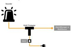
Connect the siren to one of the connections on the RJ45 T-adapter. In addition, connect the supplied KIO2 power adapter to the RJ45 Tadapter and connect the plug-in power supply unit to it. Connect the RJ45-T adapter to an AlarmManager or MultiSensor (system socket). For information on setup, please refer to docs.kentix.com
