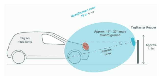
Distance from the barrier: Approx. 2 m in front of the barrier, on a post or similar near the road. The vehicle reaches the detection area earlier during the approach. Thus, the barrier will be opened a little earlier to allow smoother passage.
