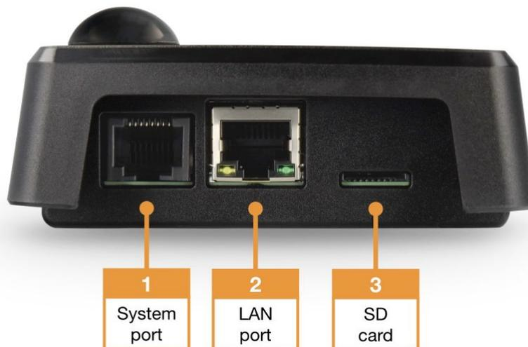
System components such as leakage sensors, door contacts, sirens or external alarms from UPS or air conditioning units can be connected via the Kentix system port (type A) of the MultiSensor. With the MultiSensor-RF, the power is also supplied via the system port (type A).
