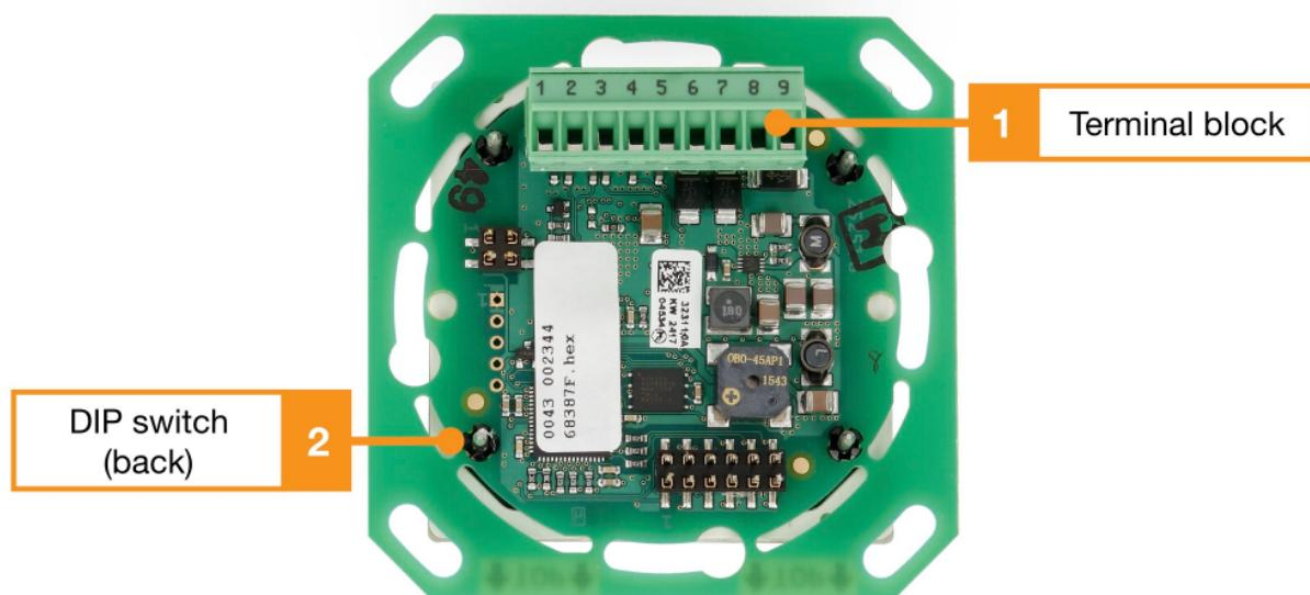
1. Terminal block 1, see wiring diagram
