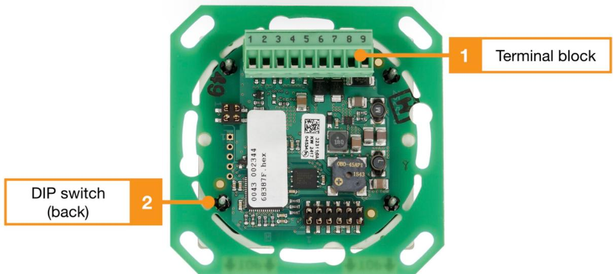
1. Terminal block 1, see wiring diagram
