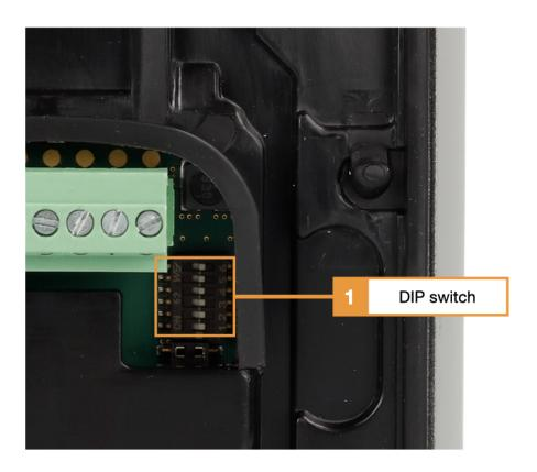
1. DIP switch for configuring the address
