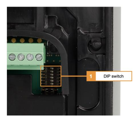
1. DIP switch for configuring the address
