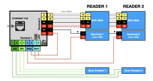
Wiring diagram AccessManager KXP-2-RS with 2x wall reader, 2x door opener, 2x door contact
