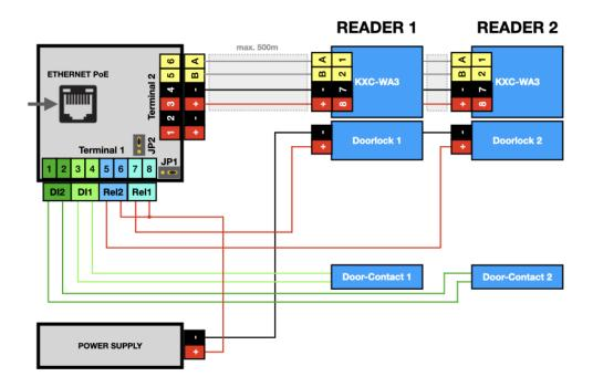
Wiring diagram Access Manager KXP-2-RS with 2x wall readers and external power supply for the door openers
