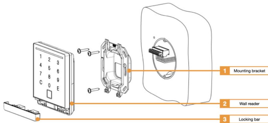
1. Mounting bracket for flush-mounted application (included in scope of delivery)
