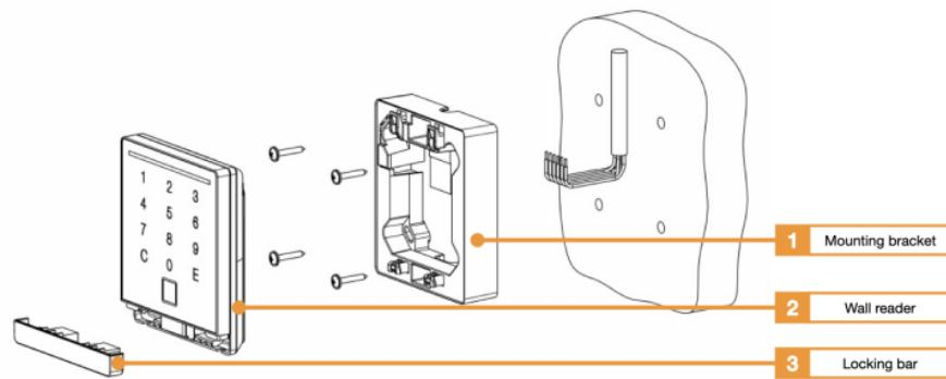
1. Mounting bracket for surface-mounted applications KXC-WA3-SMC
