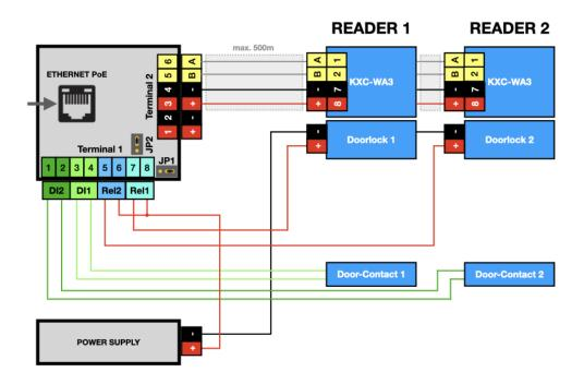
Wiring diagram Access Manager KXP-2-RS with 2x wall readers and external power supply for the door openers
