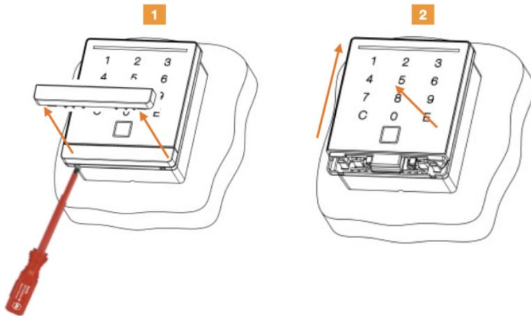
1. Insert the screwdriver into the unlocking openings and unlock the lock. Pull out the locking bar.
