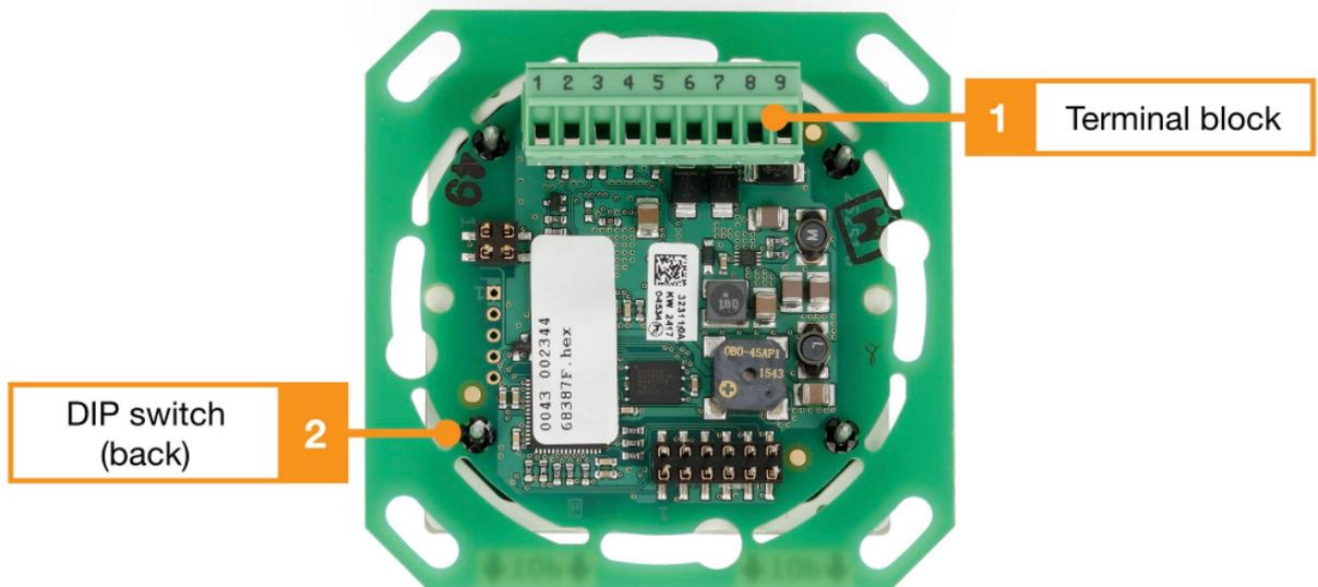
1. Terminal block 1, see wiring diagram
