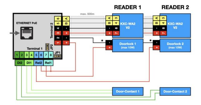
Terminal 2 on the AccessManager provides communication via the data bus and the supply of operating voltage for the wall readers. (terminals 3-6). Terminal 2 serves as a common potential for the power supply of door openers with the PoE supply voltage of the AccessManager.
