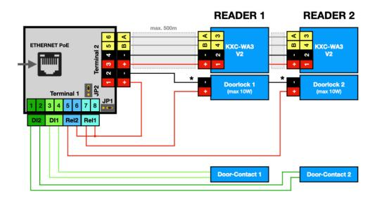
Terminal block 2 on the AccessManager (bus) is used for communication (terminals 5 and 6) and for supplying power (terminals 3 and 4) to the wall readers.
