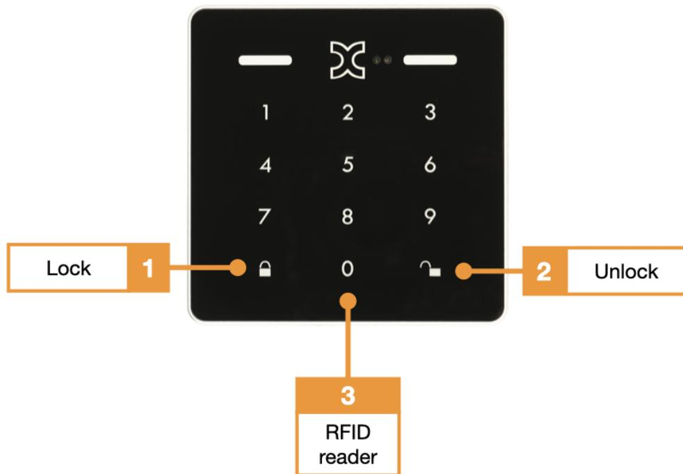
1. Touch keyboard with illuminated keypad and “arm alarm” function key
