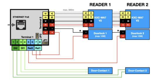
The connection example schematically shows the wiring of two DoorLock-WA7 with door contacts and external electric strikes to an AccessManager.
