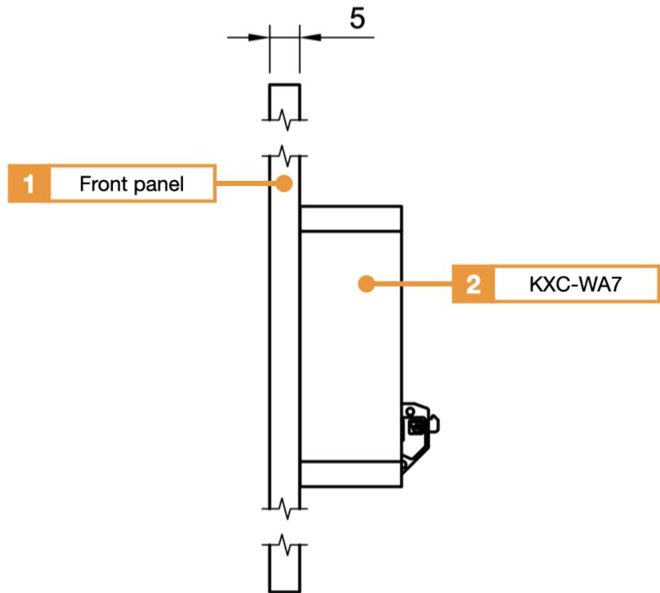
1. Front panel (maximum thickness 5mm)
