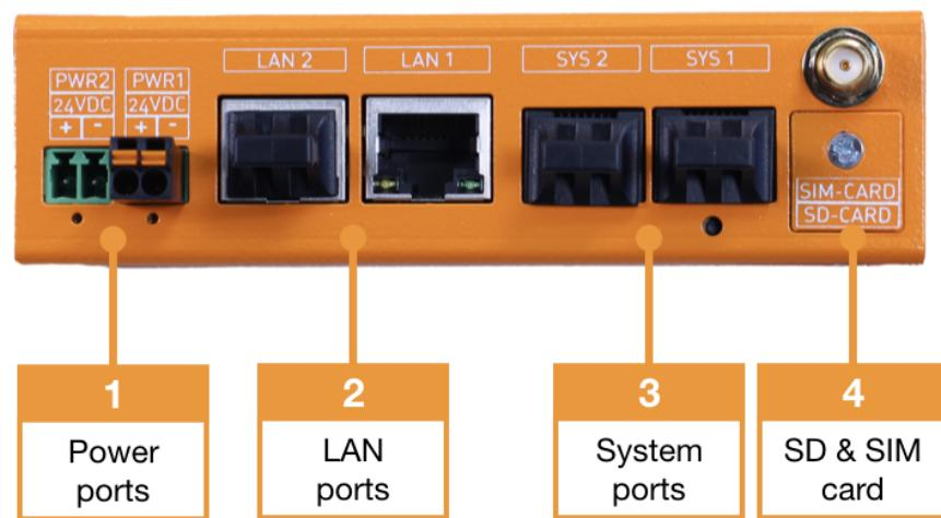
1. Connection 1 and connection 2 for the power supply (24VDC) of the Kentix SiteManager
