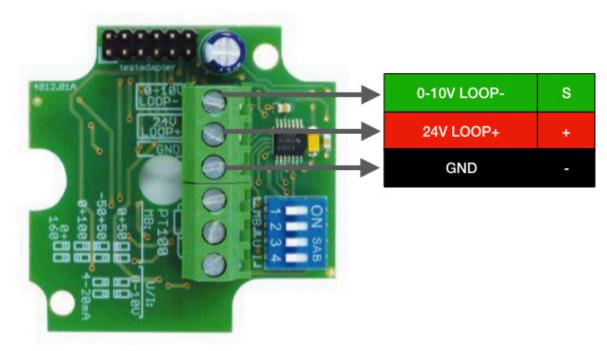
Connections and DIP switches with open housing
