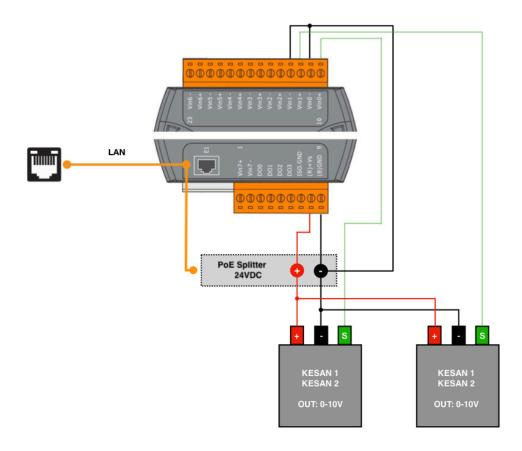
The voltage output of the PoE splitter supplies both the KIO7017 module and the two KESAN1/2 sensors with voltage. Note the performance data of the PoE splitter (min. PoE Class 3) and its general operation. We recommend to set 24VDC as output voltage at the PoE splitter if possible.
