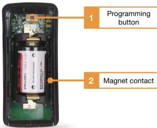
1. Teach-in key: This key is used to teach the device into the wireless network. To teach-in the sensor, start the teach-in process in the web interface of the manager and then press the teach-in button for 3sec. Press until a signal tone is heard
