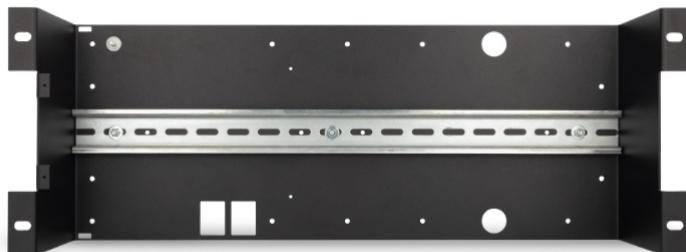
19" mounting frame with 4U for mounting up to 22 modules (TE) on DIN rail (35mm), height: 176mm, material: sheet metal 2mm, scope of delivery: 19" frame
