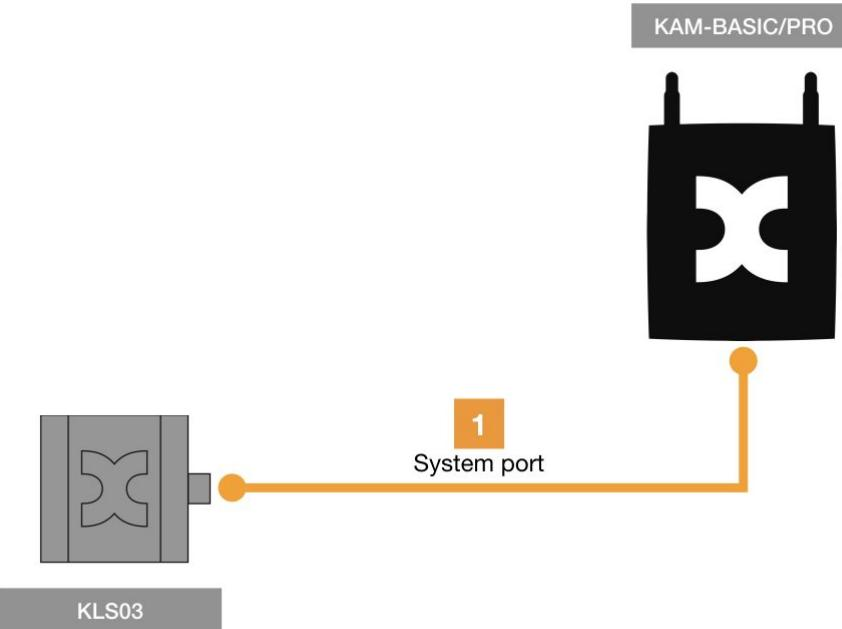
Leakage sensor on AlarmManager or MultiSensor
