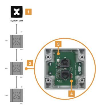
Cascading of the leakage sensors
