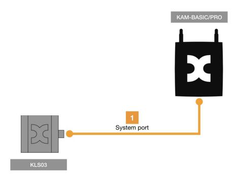
Leakage sensor on AlarmManager or MultiSensor
