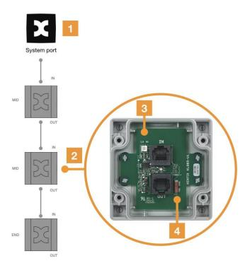
Cascading of the leakage sensors
