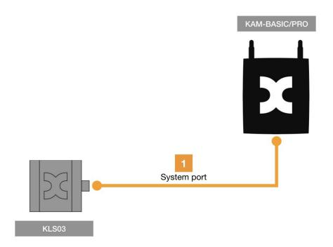
Leakage sensor on AlarmManager or MultiSensor
