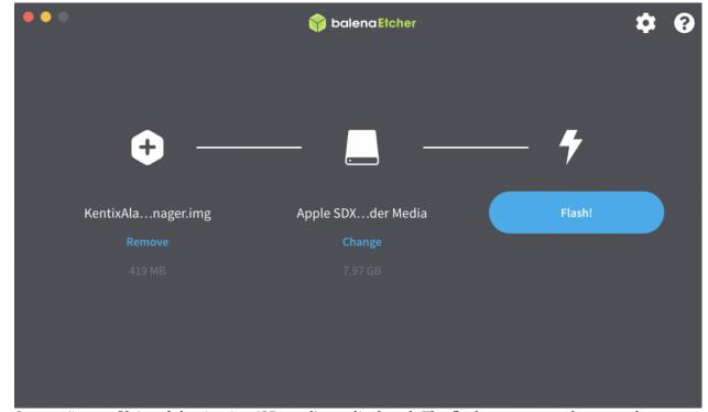
Source (image file) and destination (SD card) are displayed. The flash process can be started
