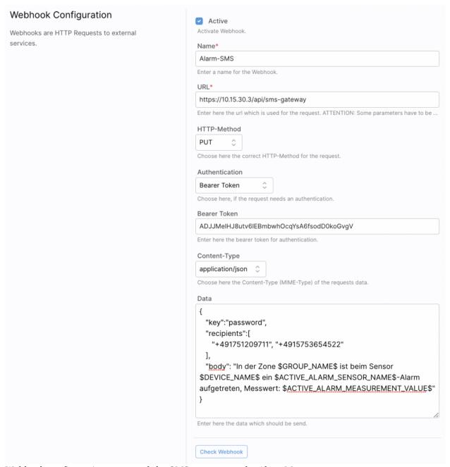
Webhook configuration to control the SMS gateway at the AlarmManager
