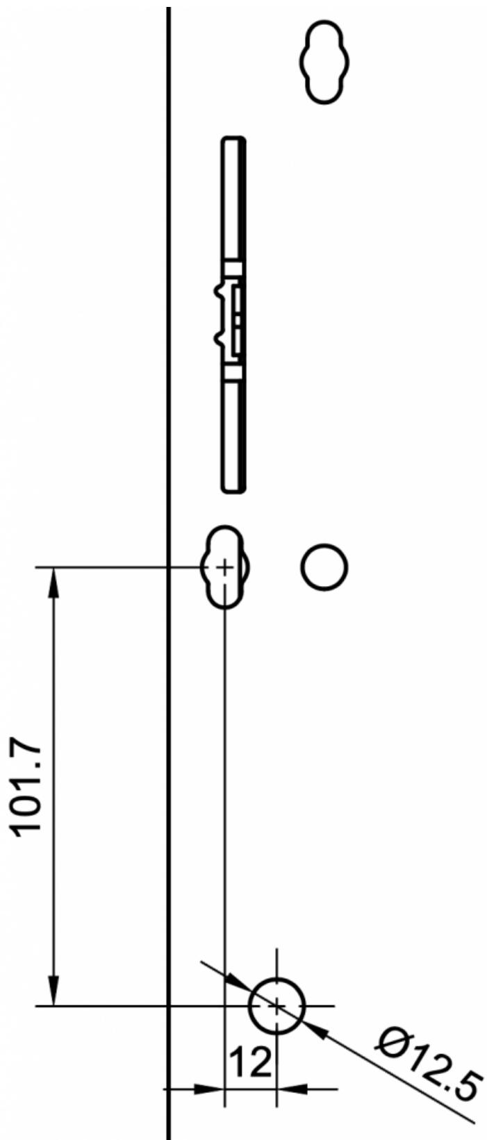
The hole pattern above is required for mounting the DoorLock-RA4 on a door. A hole of at least 12.5 mm must be drilled in the door so that the connection cable can be fed through the door.
