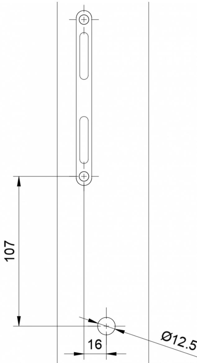
The hole pattern above is required to install the DoorLock-RA4 on a right-hinged door. A hole of at least 12.5 mm must be drilled in the door so that the connection cable can be fed through the door. If the door is hinged on the left, the position of the hole must be mirrored.
