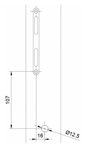
The hole pattern above is required to install the DoorLock-RA4 on a right-hinged door. A hole of at least 12.5 mm must be drilled in the door so that the connection cable can be fed through the door. If the door is hinged on the left, the position of the hole must be mirrored.
