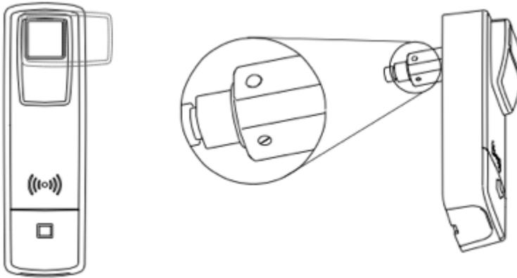
Screw in from below. Opening by turning the operating lever to the right.
