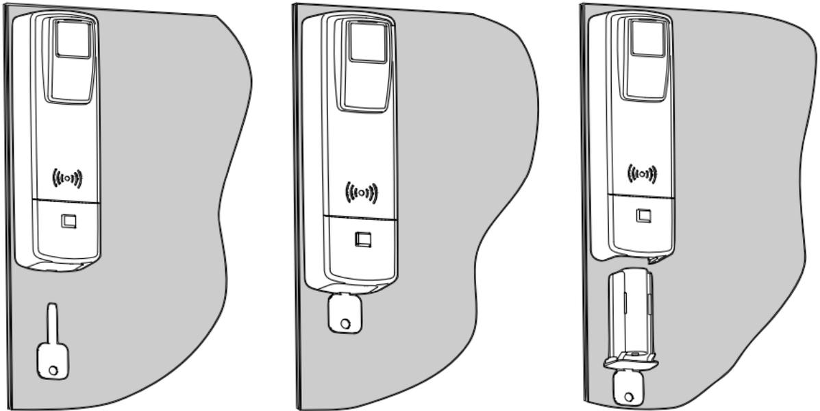
Remove the used battery and insert a new one, paying attention to the polarity.
