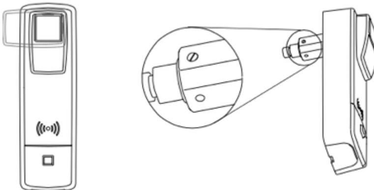
Screw screwed in sideways. Opening by turning the operating lever to the left.
