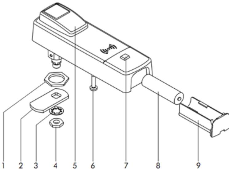
1. Fastening nut for the cabinet lock on the door
