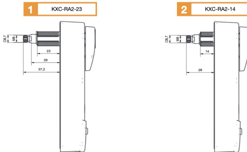
1. DoorLock-RA2-23 with a 23 mm long locking bolt
