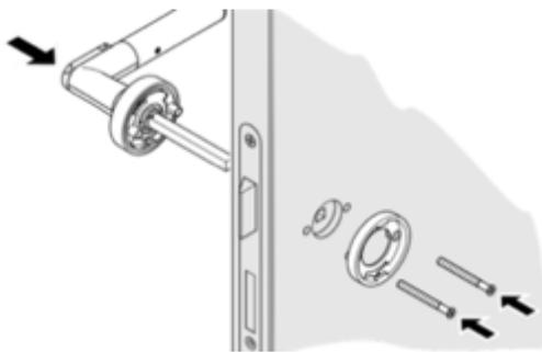
The enclosed screws are designed for doors with greater door thickness. Before screwing, be sure to check whether the screws need to be shortened so as not to damage the rosettes!
