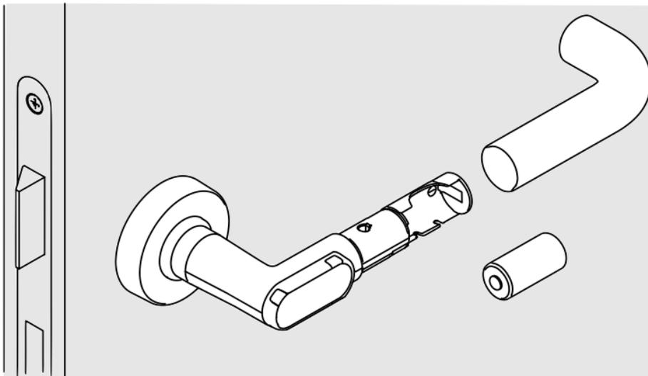
Remove the used battery and insert a new one, paying attention to the polarity. The negative pole of the battery points in the direction of the handle sleeve. When inserting the battery, the DoorLock must be in the horizontal home position.
