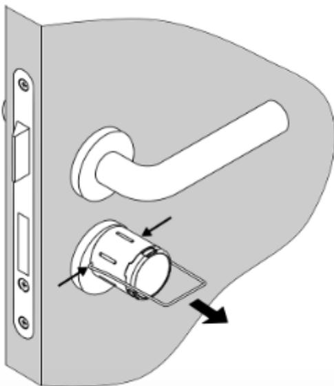
Remove used batteries and insert new batteries, paying attention to polarity.
