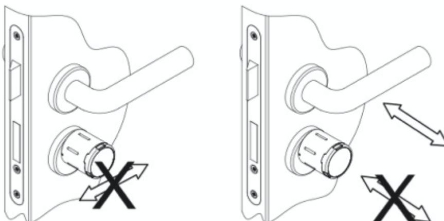
During operation, it must be ensured that, apart from the intended operation, no lateral or other external forces act on the radio knob cylinder. Likewise, the door must not be pulled
