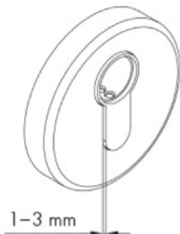
If the radio door knob and cylinder were not supplied assembled, one or two drops of a resin-free oil (ORDER-CODE: KXC-PLS50M) must be added to the cylinder body during initial installation before mounting the knob module. It must not be sprayed directly into the cylinder body with the spray can. For the DoorLock-DC BASIC radio door knob, apply an additional 1 drop of resin-free oil directly to the mechanical slider.
