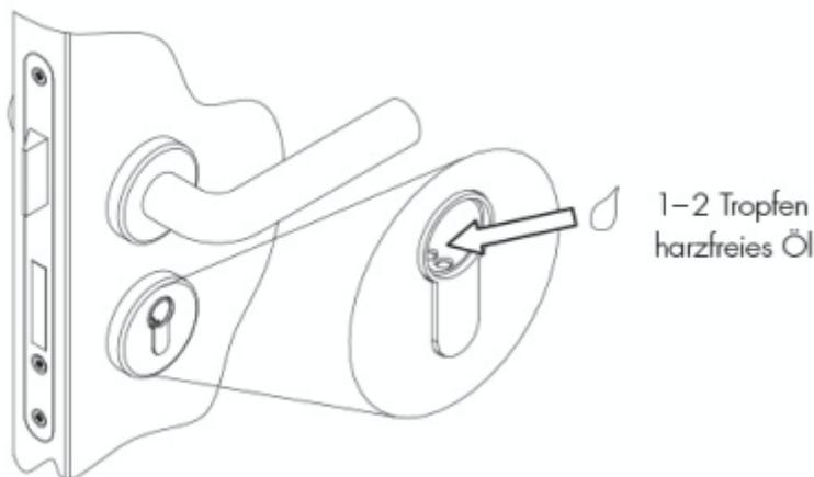
Do **not** use contact or cleaning sprays such as WD40 for maintenance.
