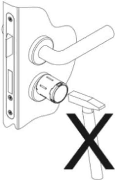
During installation, no external forces may act on the radio door knob and/or the cylinder body.
