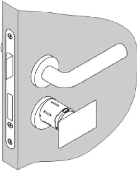
Simultaneously press in the now unlocked case locking pins of the knob module with the battery replacement tool and pull off the case.
