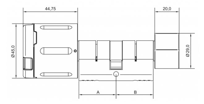
The lengths A and B are different depending on the cylinder required. To find out which cylinder lengths to use, the following guide can be used: Correctly measure locking cylinder
