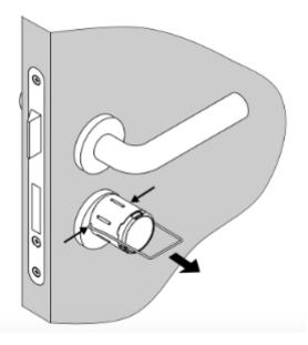
Remove used batteries and insert new batteries, paying attention to polarity.
