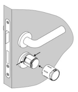
After the battery change, the knob module is still in the battery change position. By presenting the battery replacement card or an authorized key again, the knob module moves back to the home position.
