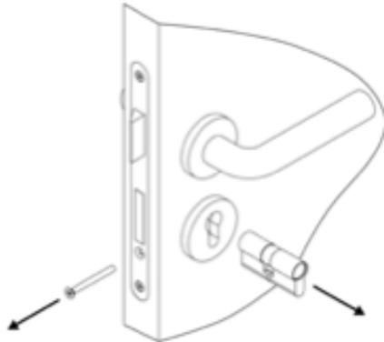
**Remove the faceplate screw and pull the existing cylinder out of the door.**
