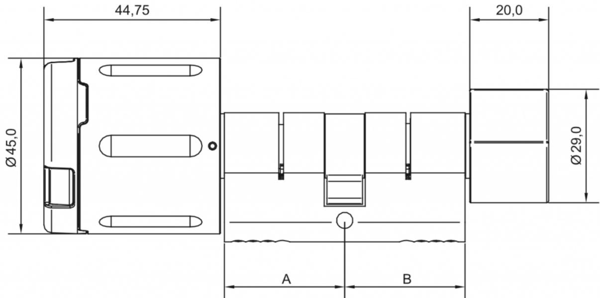
The lengths **A** and **B** are different depending on the cylinder required. To find out which cylinder lengths to use, the following guide can be used: [Correctly measure locking cylinder](#)
