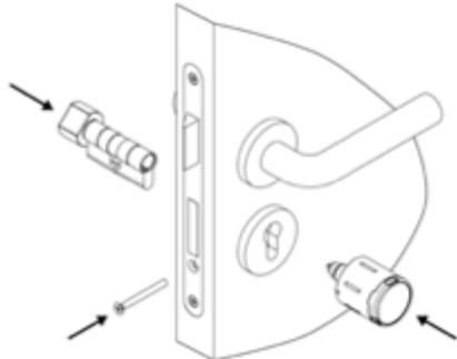
Insert the Kentix profile cylinder into the door. Then insert and tighten the forend screw.
