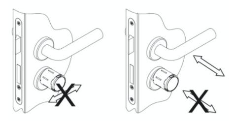
During operation, it must be ensured that, apart from the intended operation, no lateral or other external forces act on the radio knob cylinder. Likewise, the door must not be pulled open on the radio door knob. Operating the door via the radio knob results in increased stress and premature
