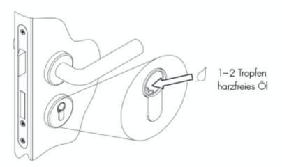
Do **not** use contact or cleaning sprays such as WD40 for maintenance.
