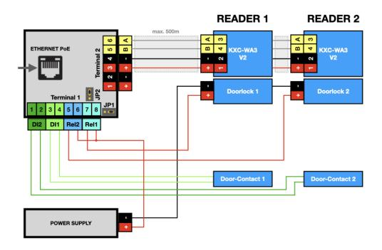
Wiring diagram AccessManager with external power supply for the door openers
