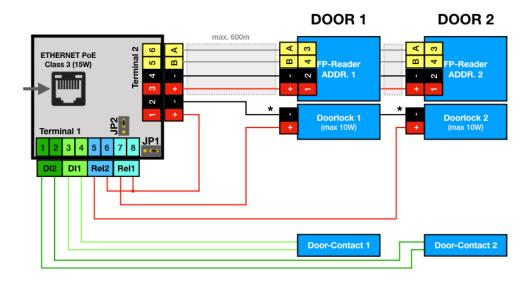
Wiring diagram AccessManager with 2x wall reader, 2x door opener, 2x door contact
