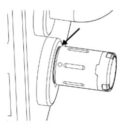
Place the battery replacement tool on the marking of the knob casing and push it together onto the knob as far as it will go. Then remove the battery replacement tool from the knob shell and test that it is firmly seated on the knob by pulling on the knob shell.
