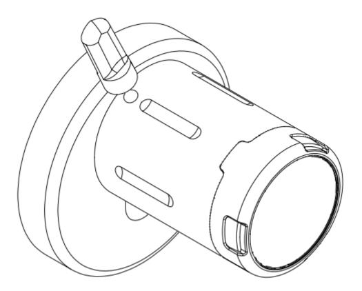
With the battery replacement tool in place, pull off the knob casing.
