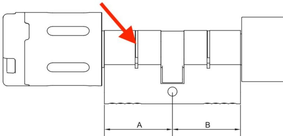
After disassembly of the DoorLock, the internal components in the cylinder can become loose and fall out.
