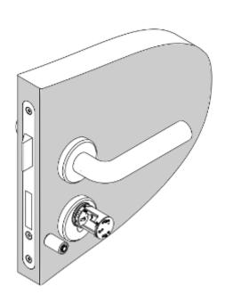
Push the knob casing onto the knob as far as it will go so that the marked point on the knob casing is aligned with the protruding plastic part on the knob.
