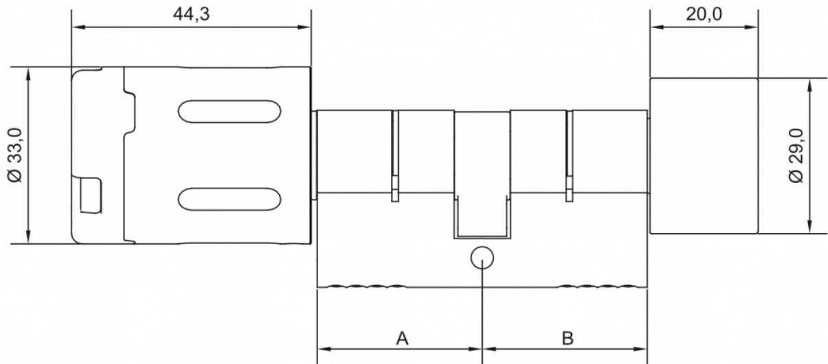
The lengths **A and B** are different depending on the cylinder required. To find out which cylinder lengths to use, the following guide can be used: [Correctly measure locking cylinder](#)
