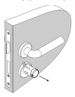
Remove the used battery and insert a new one, paying attention to the polarity.
