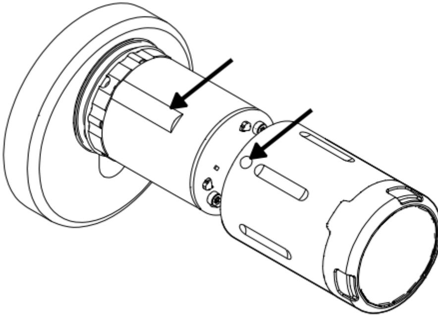
The knob casing must be pushed on so far that only the rubber seal is visible. If this is not the case, hold the knob and turn the knob sleeve slightly back and forth on the knob until the knob sleeve can be pushed on up to the rubber ring.
