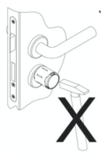
During installation, no external forces may act on the radio door knob and/or the cylinder body.
