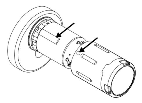
The knob casing must be pushed on so far that only the rubber seal is visible. If this is not the case, hold the knob and turn the knob sleeve slightly back and forth on the knob until the knob sleeve can be pushed on up to the rubber ring.
