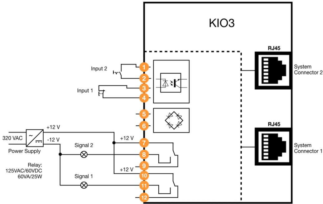
1. Terminal: Digital input 2 for potential-free wiring
